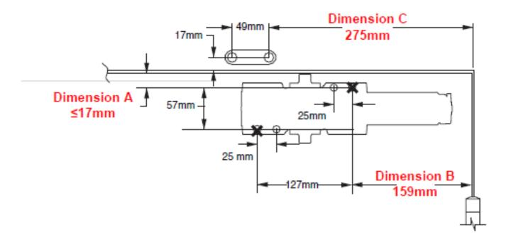
Lateral Mounting Plate Alignment – **Dimension B** aligns with the right hand most set of drilled and tapped holes, as indicated (see above). This dimension is taken from the centre line of the pivot point of the door.
