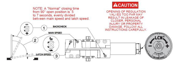
Before attempting to adjust the closer for power or speed open the door back to the maximum angle to check operation. If the door closes fully into the frame in a satisfactory manner, you do not need to make any adjustment.
