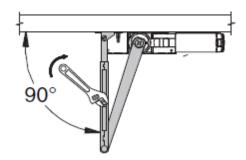
Pre-load the arm to 90° as shown - Rotate the main arm such that the fore arm meets the frame at a 90° angle. This will ensure the closer pulls the door fully into the frame once the installation is complete; providing optimum control through the closing arc.
