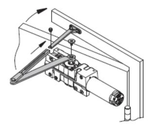
Secure the forearm with the fasteners provided. Place the closer arm hex hole onto the top of the upper pinion shaft (see below) ensuring the two marks (one on the pinion shaft and one on the arm hex hole) align correctly. Once the closer arm is in position use a rubber mallet to gently tap the arm in place fully. Use the 4040XP-159 Arm Screw – Part #4 to secure the installation.
