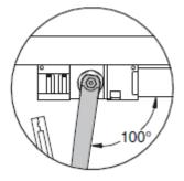
The hex hole at the end of the closer arm engages with the upper closer mechanism pinion shaft at a 100° angle to the closer
