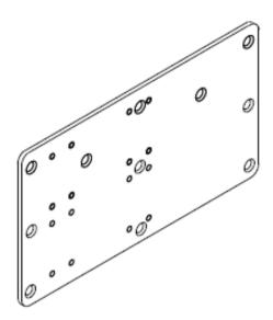
\*All fixings provided – CSK hole pattern may vary from the drawing (dictated by door detail)
